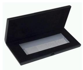
Reference test block type 2 is being used for routine assessment of the system performance of both fluorescent and colour contrast penetrant facilities and open containers. The difference of the state of action compared to the state of delivery will be shown. The test is carried out at the start of each work period.
